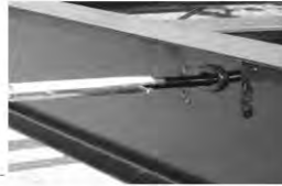
Fig. 2- Through Frame Crank Extension w/Pin
