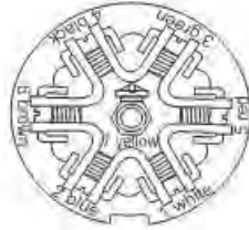
7-way trailer plug - Car end, rear view
